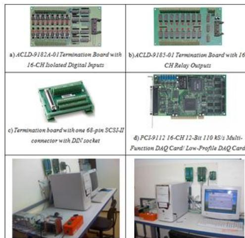
Figure 4.11: Communication Interface PCI-9112 16-CH 12-Bit 110 kS/s Multi-Function DAQ Card/ Low-Profile DAQ Card of NI Instrumentation
