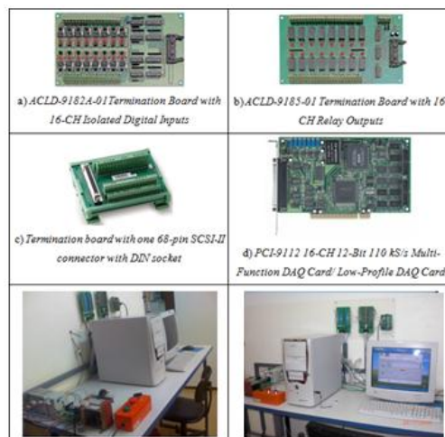
Figure 4.11: Communication Interface PCI-9112 16-CH 12-Bit 110 kS/s Multi-Function DAQ Card/ Low-Profile DAQ Card of NI Instrumentation
